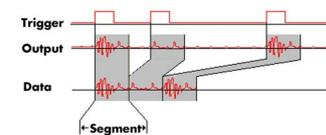
The Multiple Replay mode allows the fast output generation on several trigger events without restarting the hardware. With this option very fast repetition rates can be
