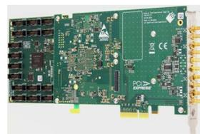
The Star-Hub is an additional module allowing the phase stable synchronization of up to 16 boards in one system. Two versions are available: one with up to 6 cards and the large version supports up to 16 cards in one system. Both versions can be mounted in two different ways, to either extend the cards length to  $\frac{3}{4}$  PCIe length occupying one slot, or extend its width to two slots whilst keeping the  $\frac{1}{2}$  PCIe length.
