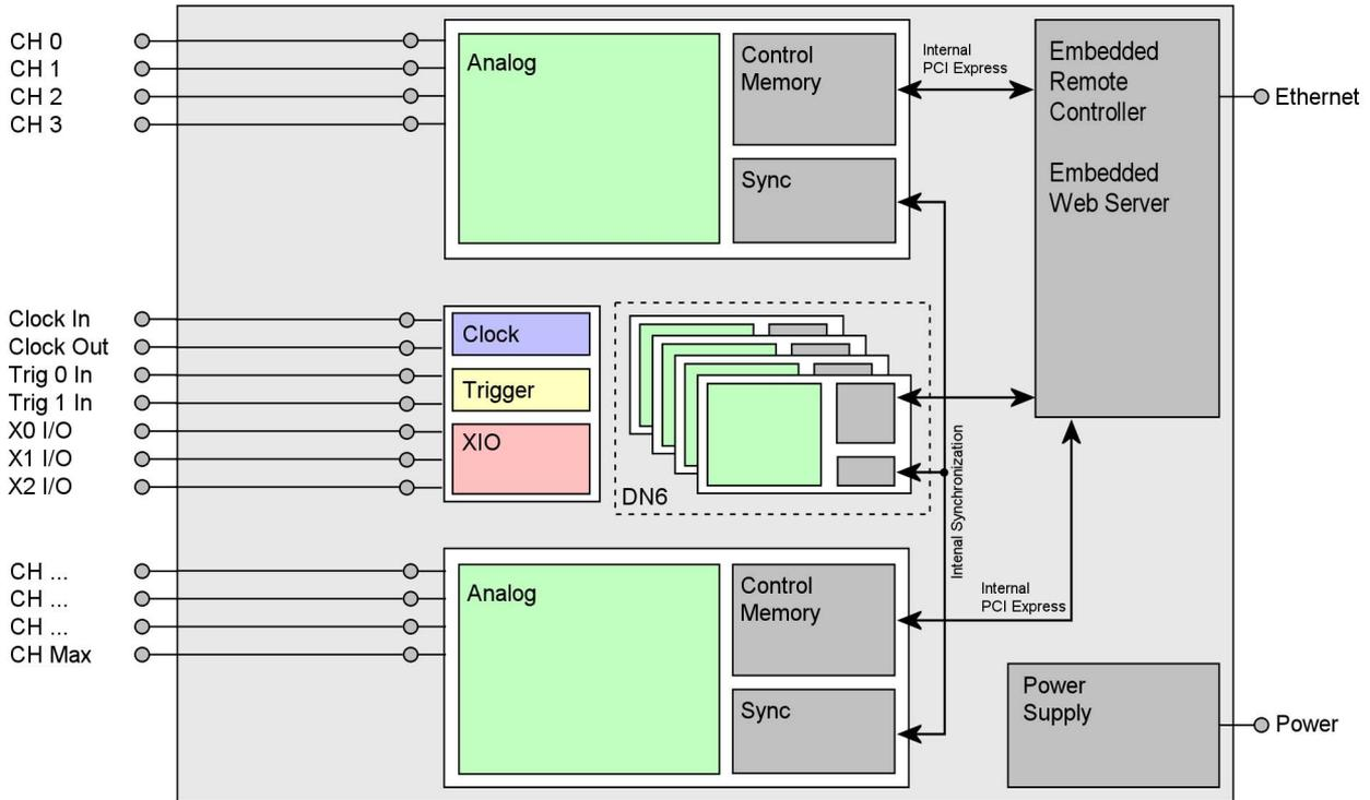
**Block diagram of generatorNETBOX module DN2.66x**
