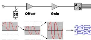
The analog inputs can be adapted to real world signals using a wide variety of settings that are individual for each channel. By using software commands the input termination can be changed
