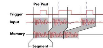
The Multiple Recording mode allows the recording of several trigger events with an extremely short re-arming time. The hardware doesn't need to be restarted in between.
