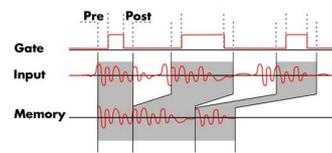
The Gated Sampling mode allows data recording controlled by an external gate signal. Data is only recorded if the gate signal has a programmed level. In addition
